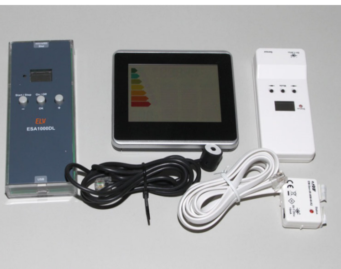
Consumption data monitor for reading electricity consumption on analogue and digital electricity meters with and without data loggers in order to create the load profile (ELV)
