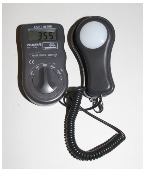
Figure 26: Illuminance meter for measuring illuminance
